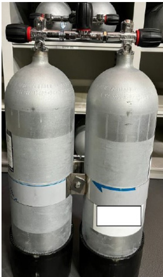
Figure 1 Two bands are required for the Thermo and XS Isolation manifolds. This picture shows only one band.
