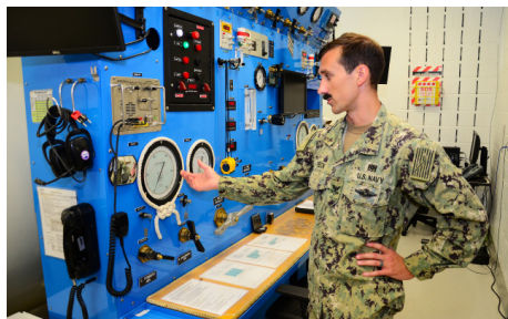
PENSACOLA, Fla. (June 14, 2022) Hospital Corpsman 2nd Class Evan Peck, a member of the Naval Aerospace Medical Institute Hyperbaric Medicine team, points out the depth gauge of the recompression chamber on Naval Air Station Pensacola, June 14, 2022. The recompression chamber is used in hyperbaric medicine, and can treat many injuries and conditions with the patient receiving oxygen or oxygen blends while in the chamber. (U.S. Navy photo by Joshua Cox)
